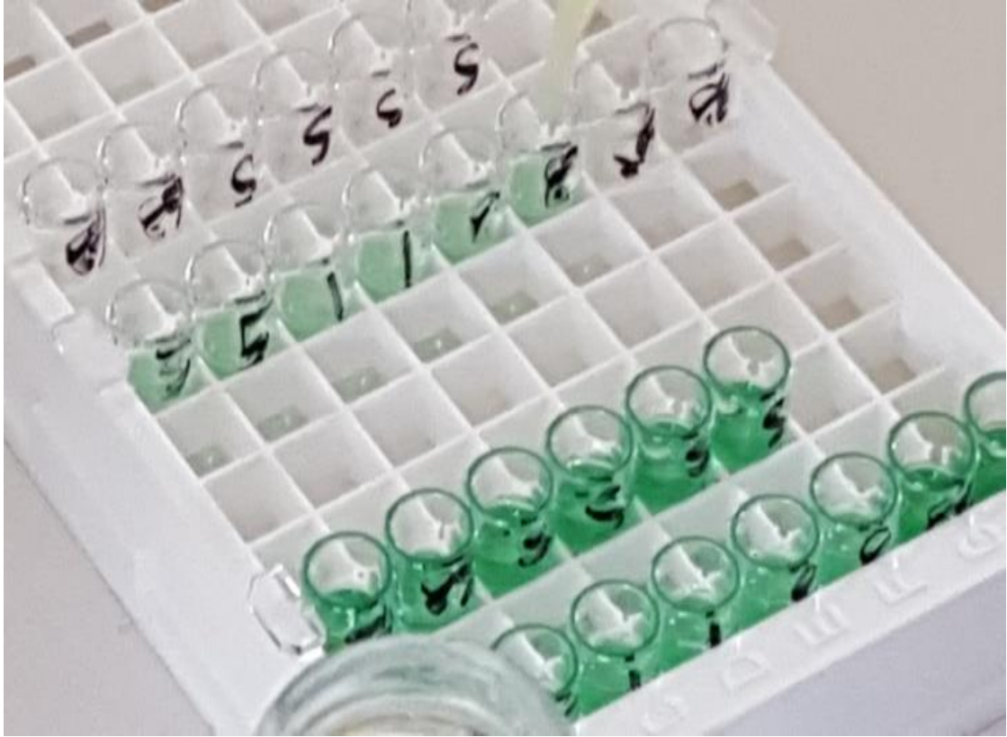
Appendix IV: Microwells with filtrate, substrate and antibody ready to be inserted into the analyzer for AFT analysis (Source: Author, 2016)
