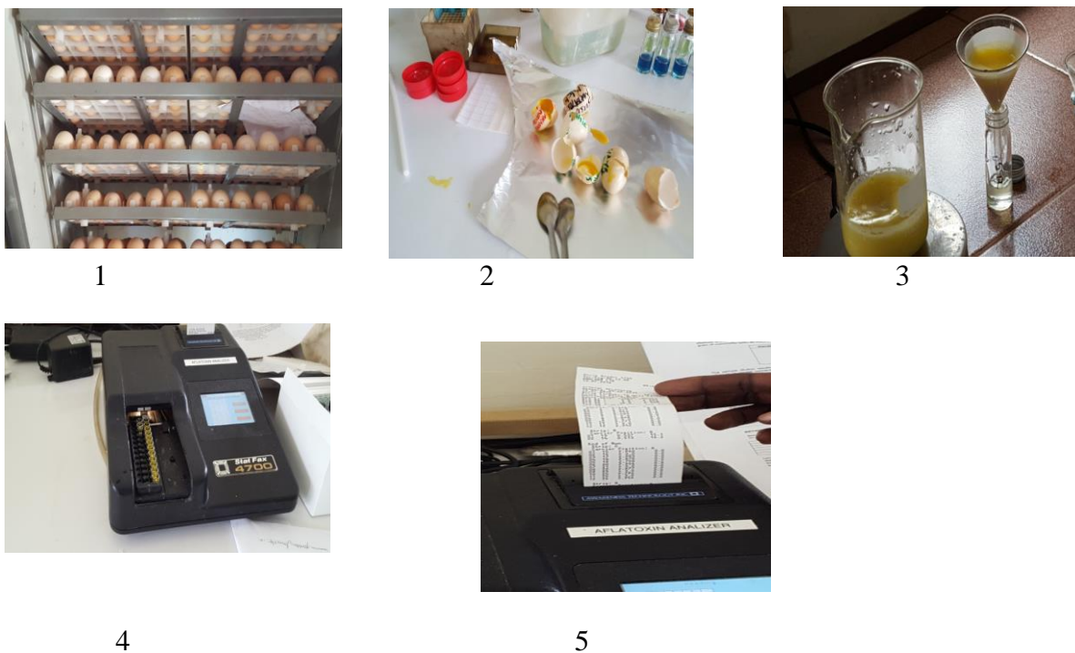
Plate 5: Egg samples are stored well in cold chamber of the fridge (1), then broken (2), contents are poured in a beaker, stirred and filtered (3). Microwells are inserted into microwell-holder in the analyzer (4) and the results are printed in a sheet of paper (5).
