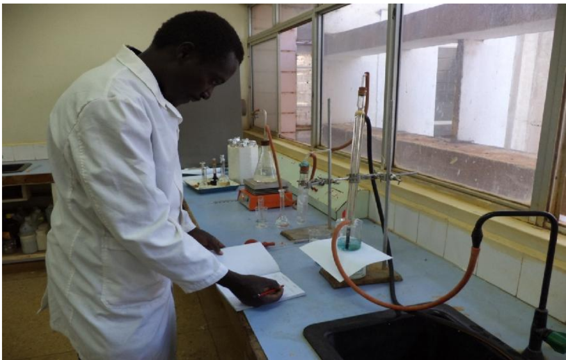
Plate 2: Back distillation during determination of crude protein, Fisheries Laboratory 1, University of Eldoret (Source: Author, 2016)
