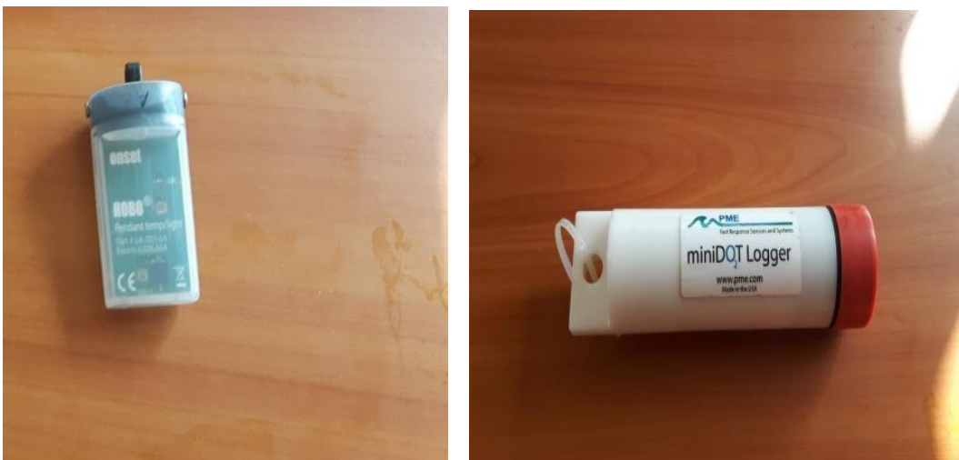
Plate 4: Light logger (left) and mini DO 2 T logger (right) (Source: Author, 2016)
