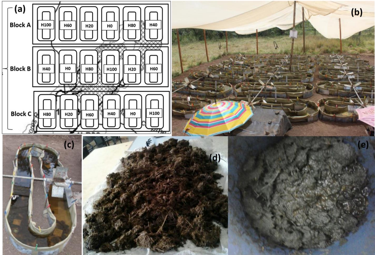
Plate 2: (a) Allocation of dung treatments in three blocks driven independently by paddle wheels (b and c) layout and details of mesocosms, (d) hippo dung, and (e) cattle dung. (Source: Author, 2016 )
