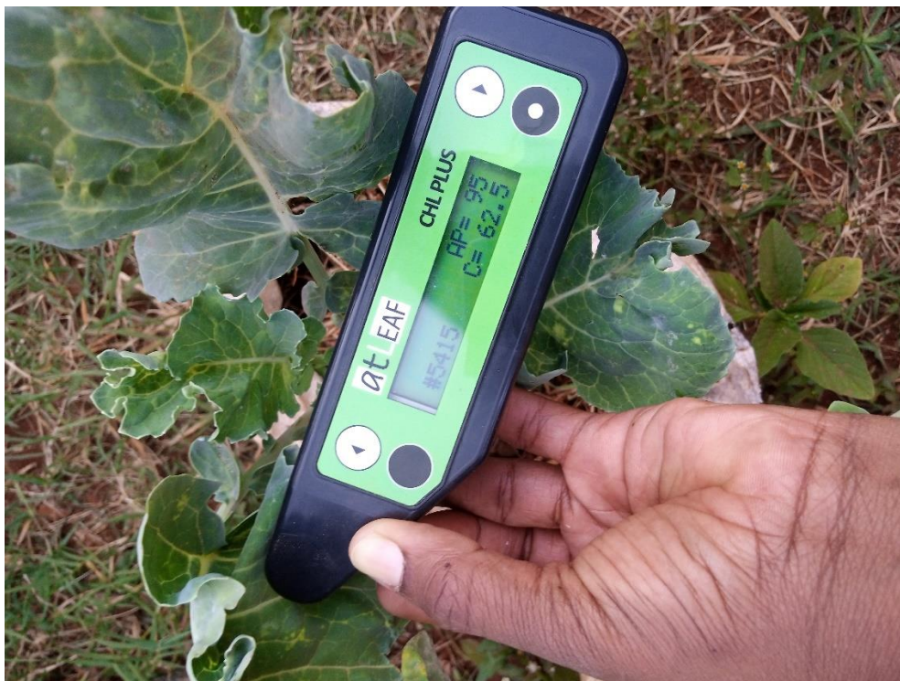
Plate 3.6: In vivo Measurement of Kales leaf chlorophyll content using atLEAF METER (Source: Author, 2021)
