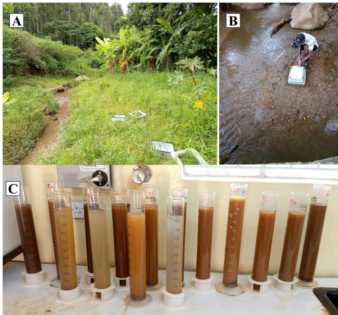
Plate VI: GHG sampling and soil analysis. Sampling in the Upland zone characterized by forest and mixed farming, with smaller streams in (A). Instream greenhouse (GHG) sampling in a Midland zone (B), and clay content analysis (C). Source: (Author 2025).
