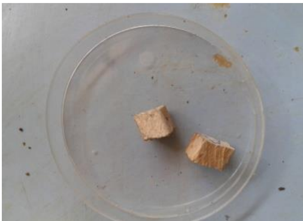
Plate 3.3 Typical cube that have been damaged by termites.
