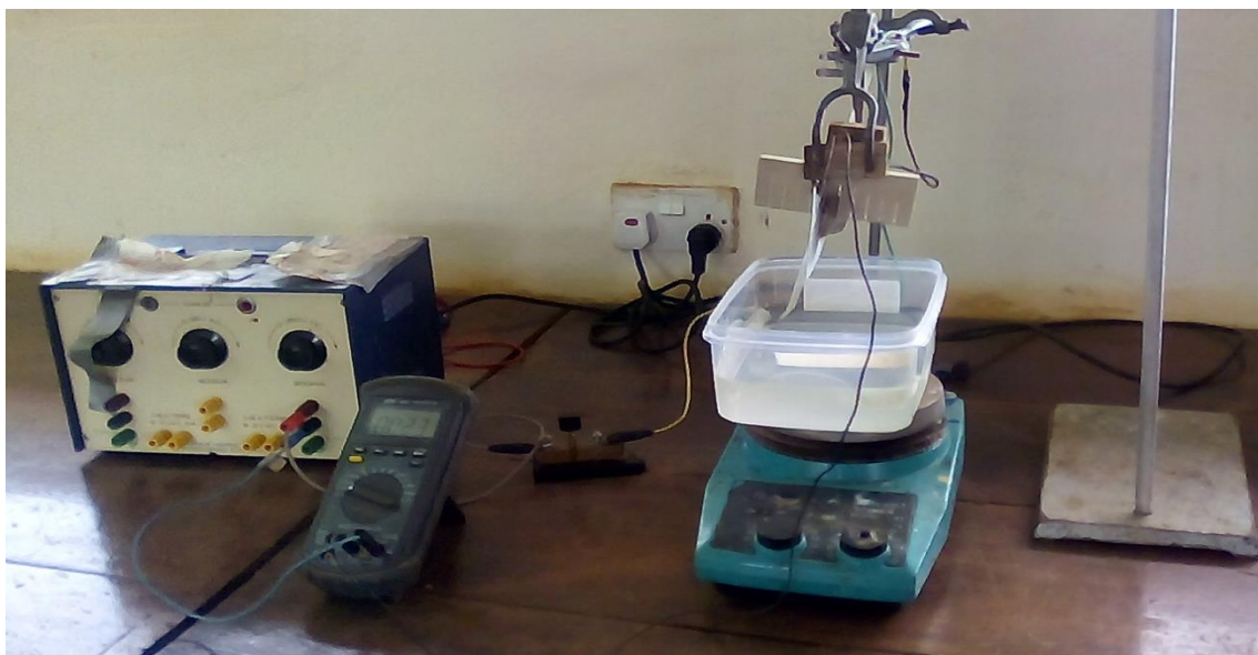
Figure 3.1: Experimental set up for anodization of TiO 2 plate. (Source : Author, 2018)
