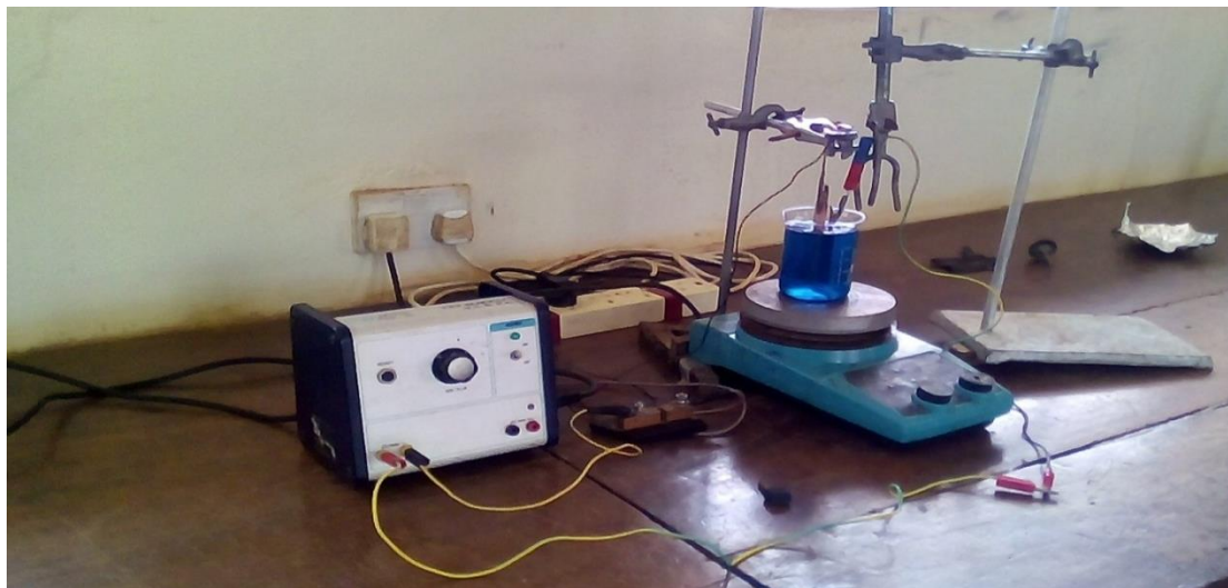
Figure 3.2: Electrodepositing set up for pigmentation. (Source: Author, 2018)
