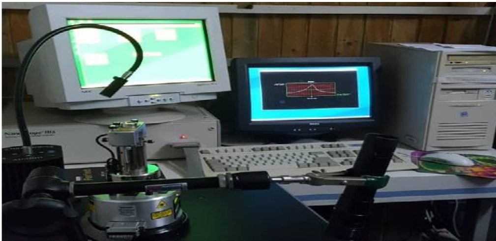
Figure 3.8: Atomic force microscopy set – up in operation. (Source: Author, 2018)
