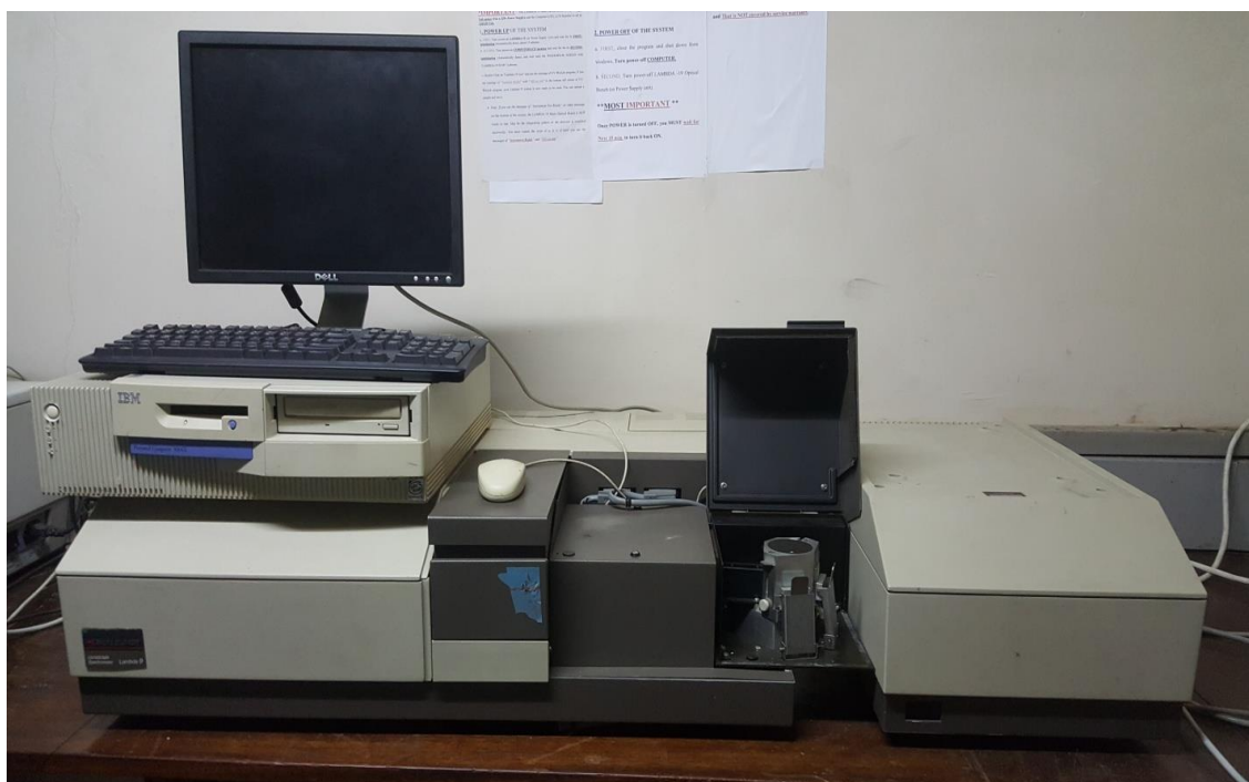
Figure 3.5: Perkin Elmer (UV/VIS/NIR Lambda 9) Photo-spectrometer set up with the Integrating Sphere accessory (Source: Author, 2018)
