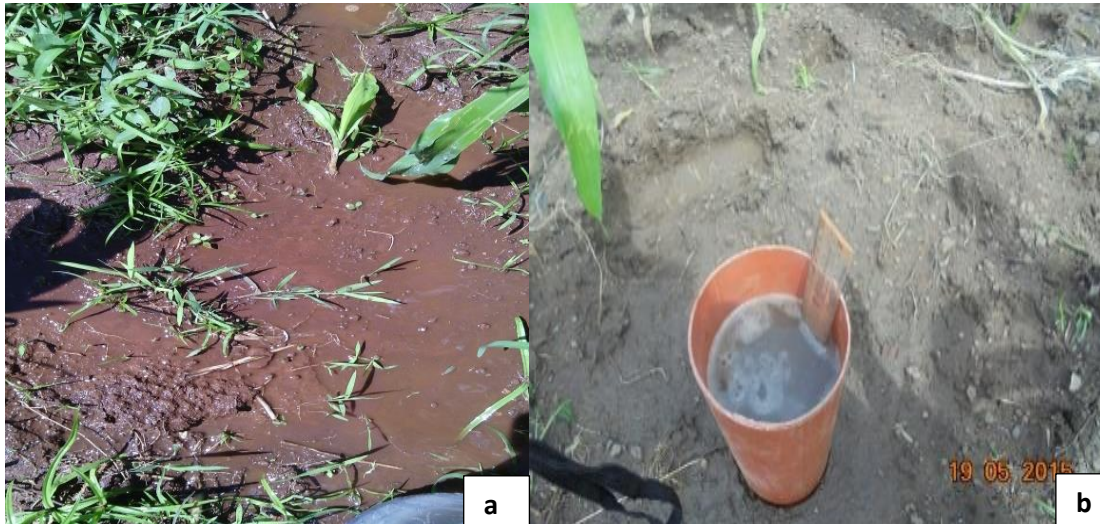
Plate 2: Demonstrations of infiltration measurement in the field using a PVC pipe to mimic single-ring infiltrometer
