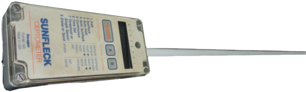
Plate 3.3: The ceptometer apparatus at the TRFK used to measure PAR in mol\ m^{-2}\ s^{-1} (Source: Author, 2012).
