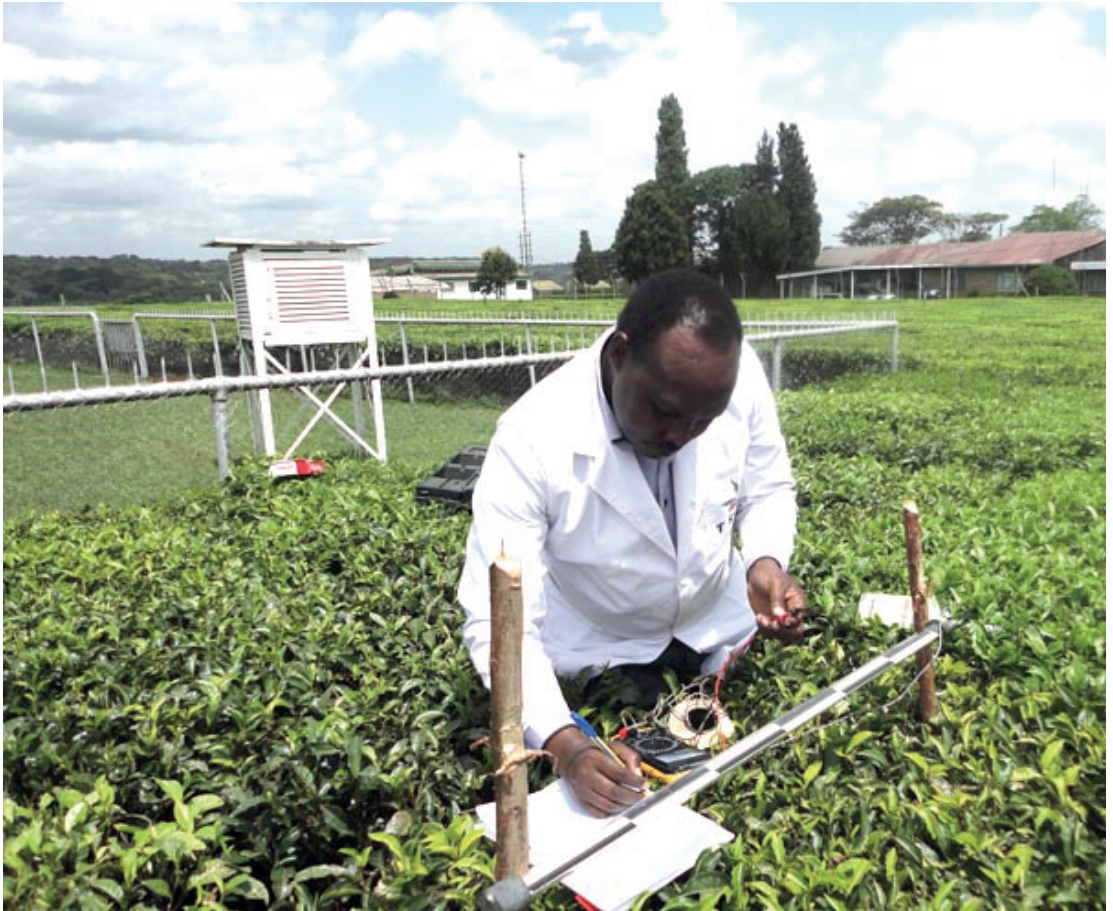
Plate 3.1: Use of tube solarimeter and voltmeter equipment to measure solar radiation reaching top of tea canopy (Source: Author, 2009).
