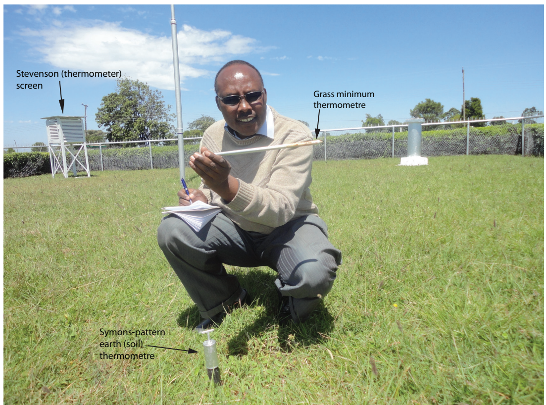
Plate 3.4: The (thermometer) Stevenson screen, Symons-pattern earth (soil) thermometer and grass-minimum thermometer (Source: Author, 2009).
