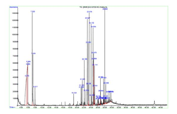
Fig 4.1. GC-MS mass spectra of bacterial volatile organic compounds of ethyl acetate extracts from *P. polymyxa* KaI245 cultures. This gave a total of 50 metabolites.
