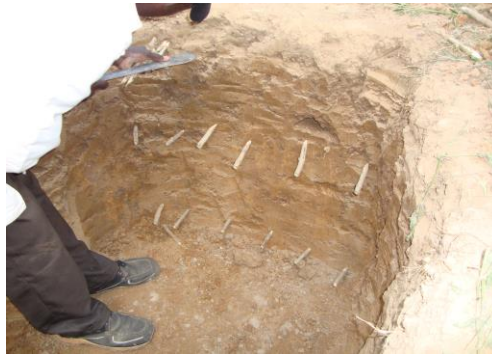
Identifying horizons in profile pit No. 4, on Owoko's farm in Got Nanga, Siaya County (Source: Author, 2010)
