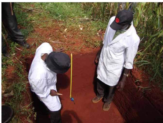
Measuring the depth a soil profile pit No. 2 on Indombela's farm Kabras, Kakamega County (Source: Author, 2010)
