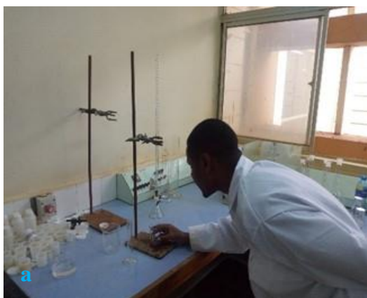
Plate 3.9: Running water samples via Cadmium column for nitrate (a) and reading the absorbance of nutrients with spectrophotometers (b) (Source: Author, 2020)
