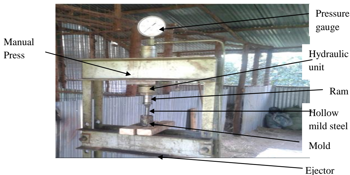
Figure 3.4: Briquetting process using manual Press
