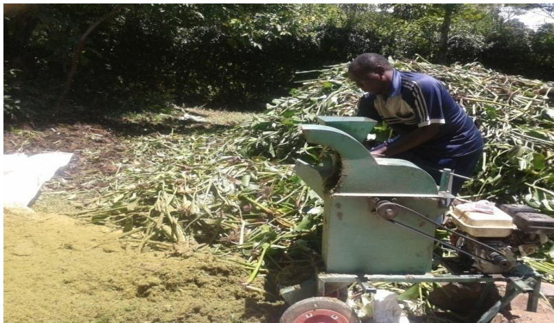
Figure 3.2: Chopping water hyacinth using shredder (From ATDC Siaya)
