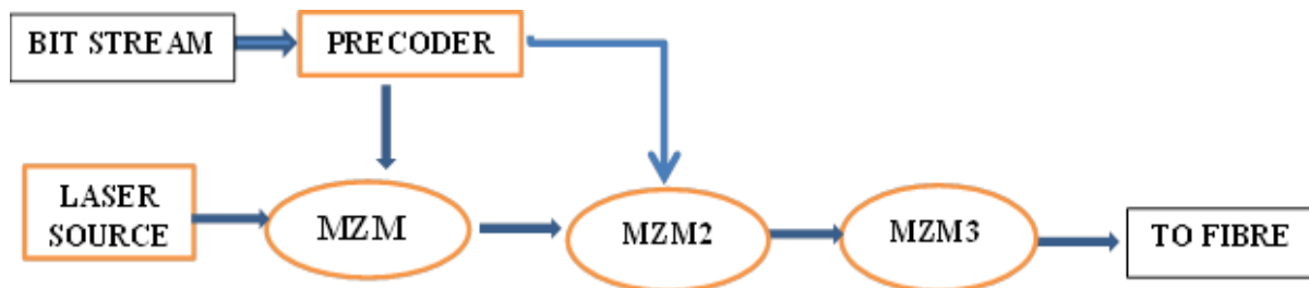
Figure 1. Transmitter configurations used in the Optisystem tool for simulation.
