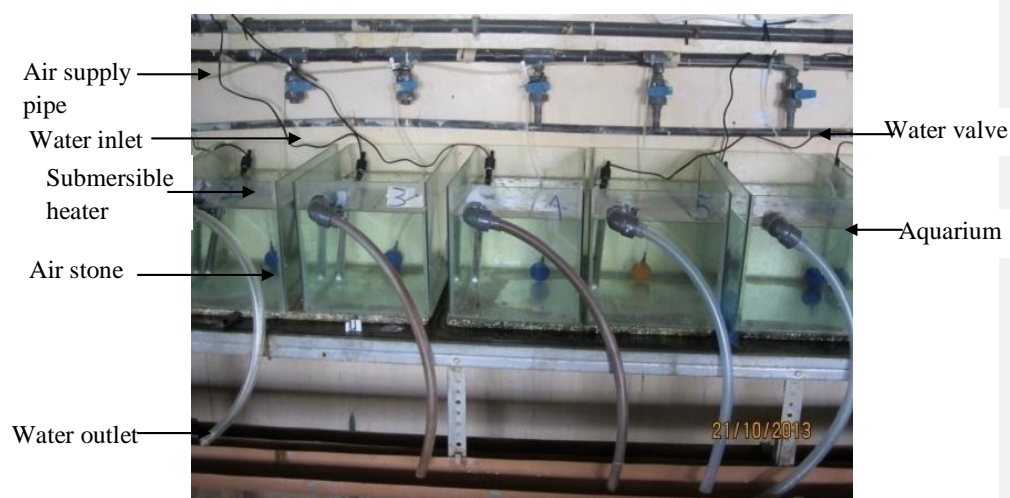
Plate 3.1: Aquaria egg incubators for L. victoriana from the four rivers. (Source: Author, 2014)
