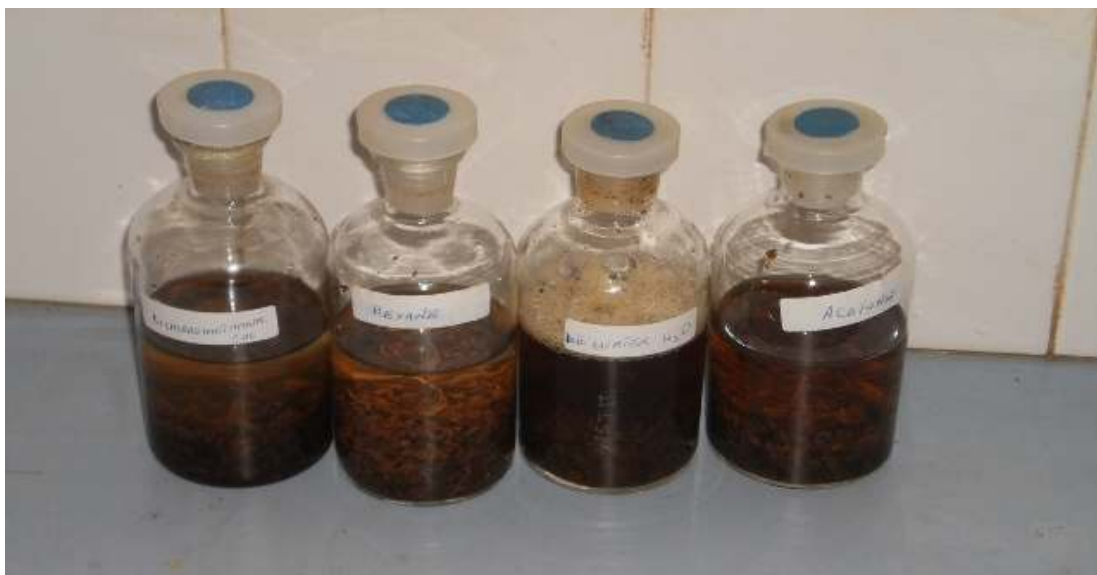
Plate 4: Extraction of A. Malacophylla wood chips by cold soaking method (Author, 2012)
