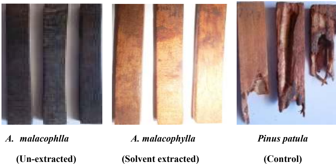
Plate 11: Extent of termite attack on wood specimens exposed in the field for six months (Author, 2012)
