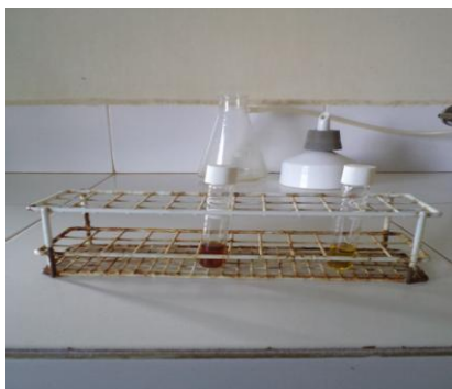
Figure 3.6: High and low range Chemical Oxygen Demand reagents ( low range: 0 – 15,000 mg/l; high range: 15,000 plus mg/l. Source: Author, 2012.
