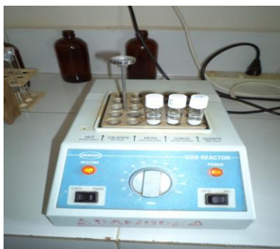
Figure 3.6: High and low range Chemical Oxygen Demand reagents ( low range: 0 – 15,000 mg/l; high range: 15,000 plus mg/l. Source: Author, 2012.
