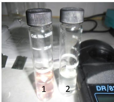
Figure 6: The HACH colorimeter (DR/820) and HACH nitrite reagents for determination of nitrites in samples (Source: Author, 2012)
