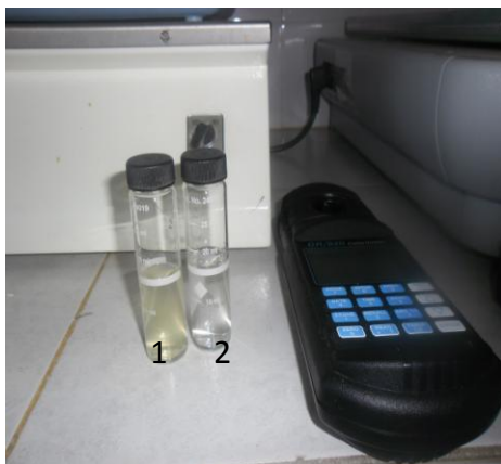
Figure 7: The HACH colorimeter (DR/820) and HACH nitrate reagents for determination of nitrates in samples (Source: Author, 2012)
