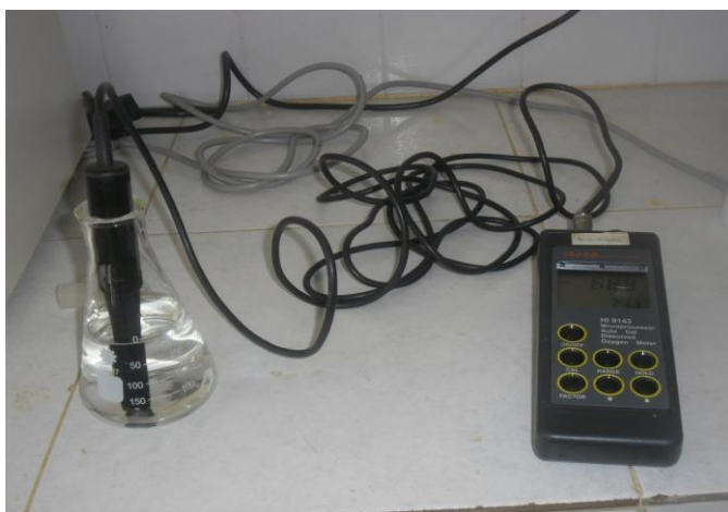
Figure 8: HANNA DO meter (HI 9143) for determination of DO in samples. (Source: Author, 2012)
