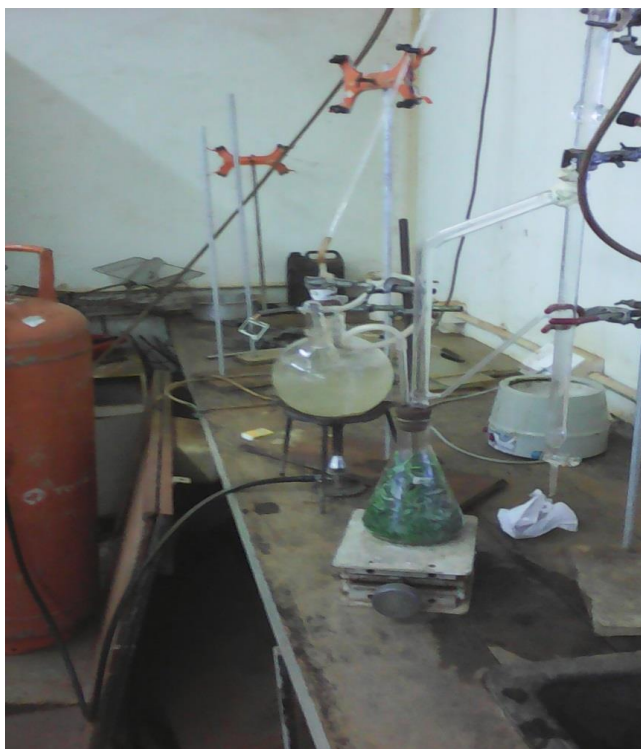
a) Picture showing steam distillation setup
