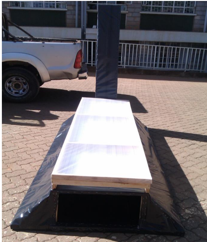
Fig. 3.3: A figure showing a prototype of the modified Horticultural Lab mixed modes solar dryer (Source: Author, 2014)
