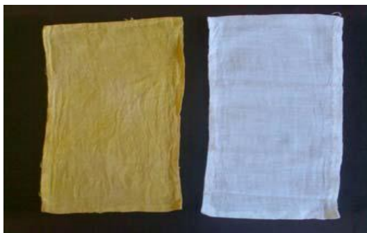
Fig. 24 a Tri-mordanted cotton fabric (bleached) article 002 dyed at 80-90 0 C. Control on the right.
