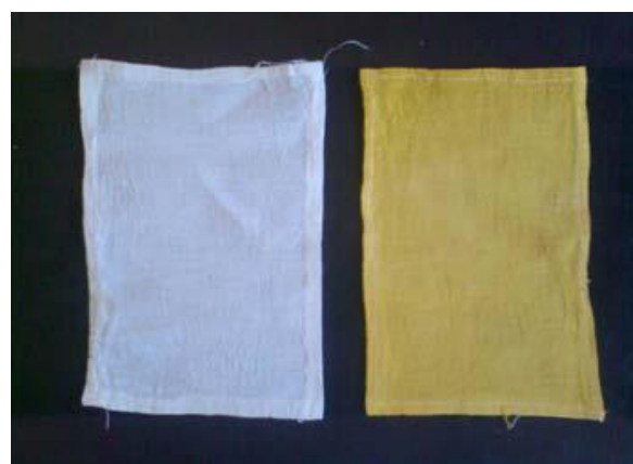
Fig. 25b Single-mordanted cotton fabric (un-bleached) article 002 dyed at 80-90 0 C. Control on the left.
