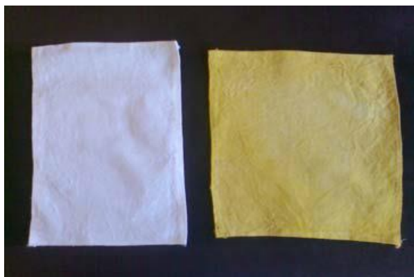
Fig.25c Single-mordanted cotton fabric (un-bleached) article 053 dyed at 80-90 0 C. Control on the right.
