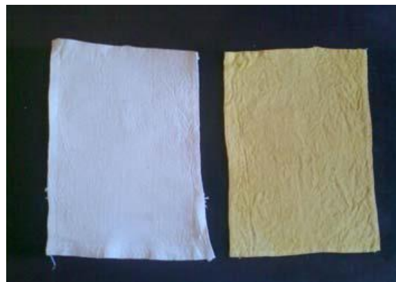
Fig. 25d Single-mordanted cotton fabric (un-bleached) article 053 dyed at 80-90 0 C. Control on the left.
