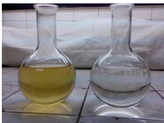
Fig .28a Resulting faint yellow alkali solution after dyed fabric for 2 minutes. Unused alkali solution on the right.
