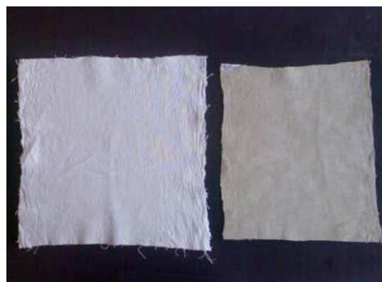
Fig. 26 b Un-bleached cotton fabric article 002 dyed at 80-90 0 C. Control on the left.
