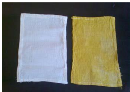
Fig. 23b Tri-mordanted cotton fabric (un-bleached) article 002 dyed at 50-60 0 c. Control on the left.
