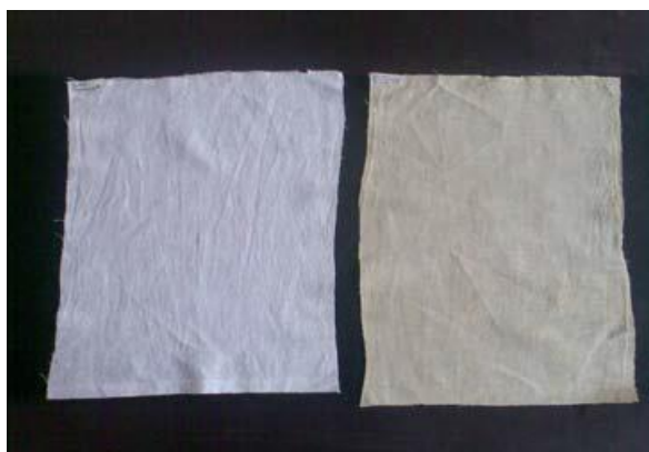
Fig. 26a Bleached cotton fabric article 002 dyed at 80-90 0 C. Control on the left.
