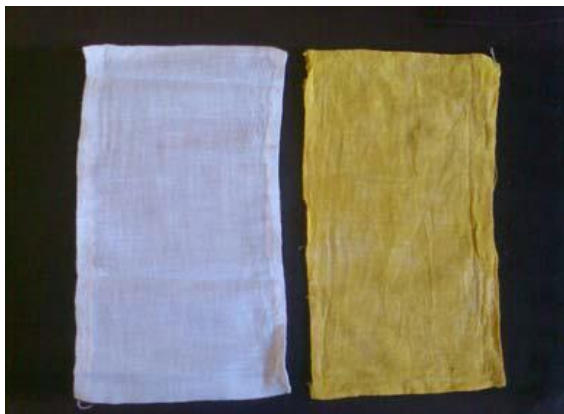
Fig. 22 a Tri-mordanted cotton fabric (bleached) article 002 dyed at rtp. Control on the left.
