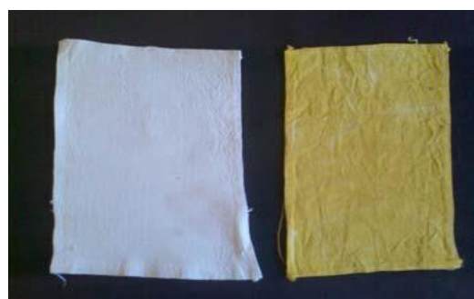
Fig. 23d Tri-mordanted cotton fabric (bleached) article 053 dyed at 50-60 0 C. Control on the left.
