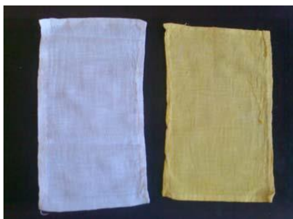
Fig. 25a Tri-mordanted cotton fabric (bleached) article 002 dyed at 80-90 0 C. Control on the right.
