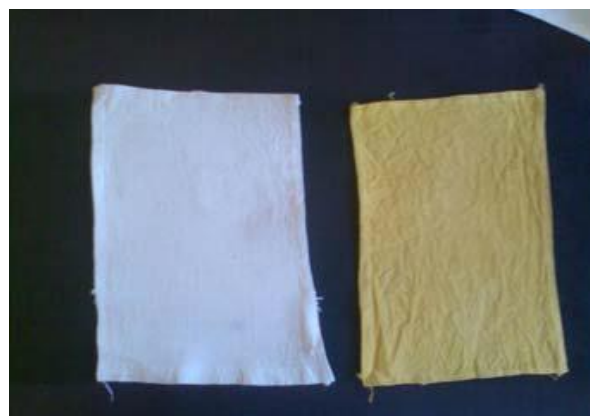
Fig. 24d Tri-mordanted cotton fabric (bleached) article 053 dyed at 80-90 0 C. Control on the left.
