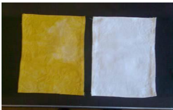
Fig.22 c Tri-mordanted cotton fabric (bleached) article 053 dyed at rtp. Control on the right.
