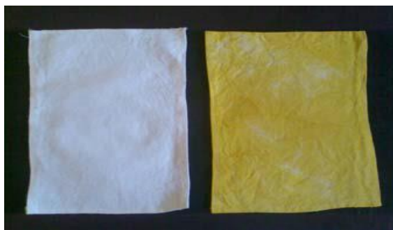
Fig. 23c Tri-mordanted cotton fabric (bleached) article 053 dyed at 50-60 0 C. Control on the left.
