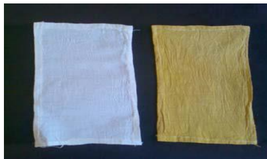
Fig. 24b Tri-mordanted cotton fabric (bleached) article 002 dyed at 80-90 0 C. Control on the left.
