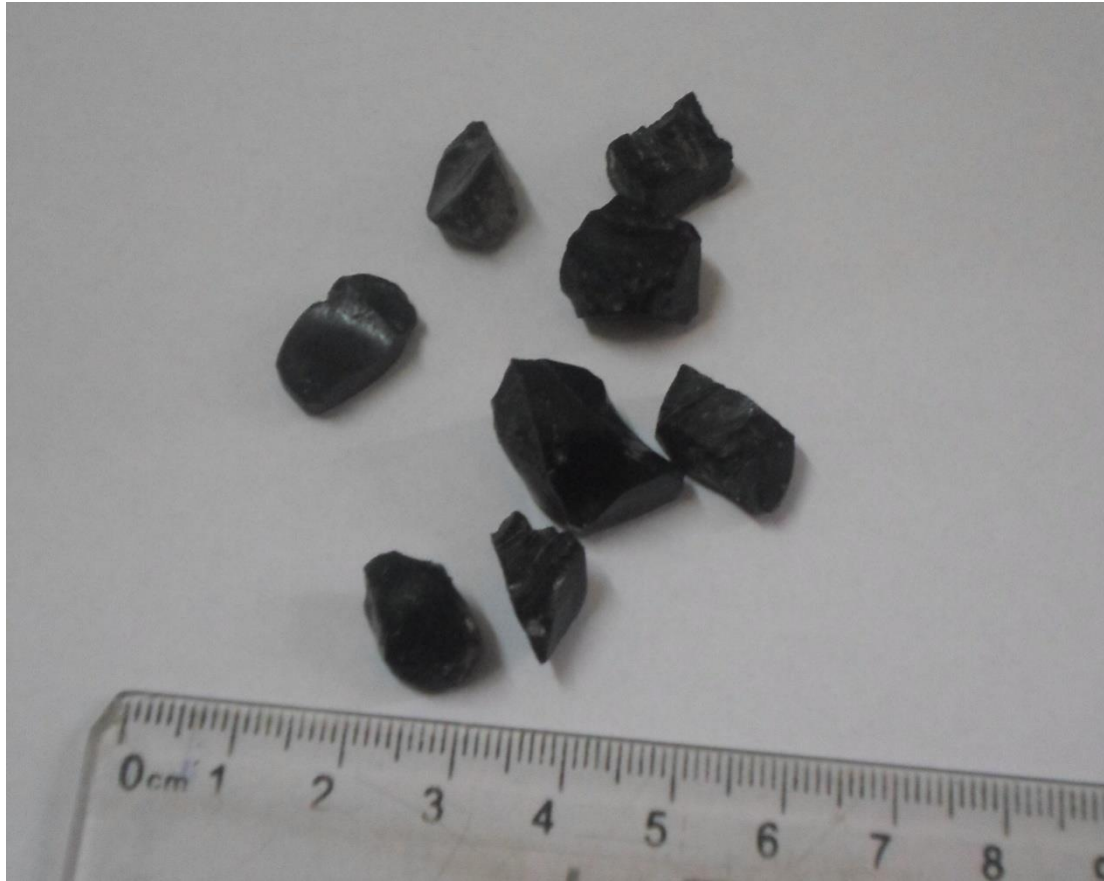
Plate 4.30: Broken obsidian particles found in the dust around Silali basin (Source: Author, 2015).
