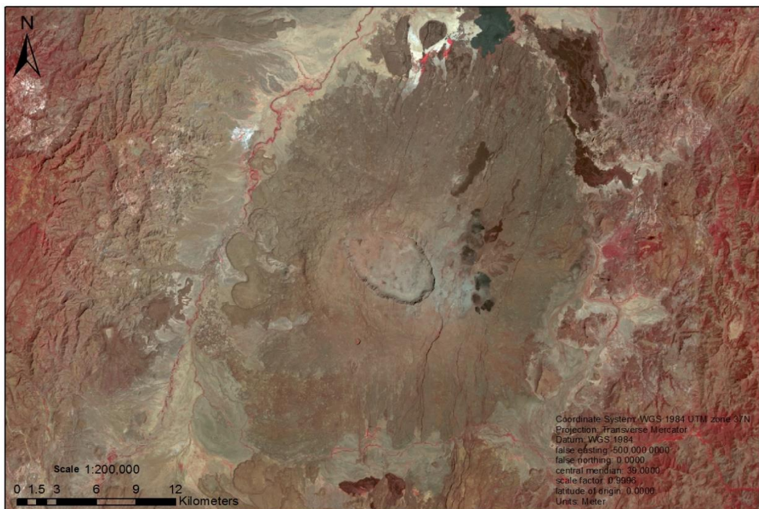
Plate 4.4: A false color image of Landsat 8, bands 5 (Red), 4 (Green) and 2 (Blue), showing the Silali basin (courtesy of RCMRD).
