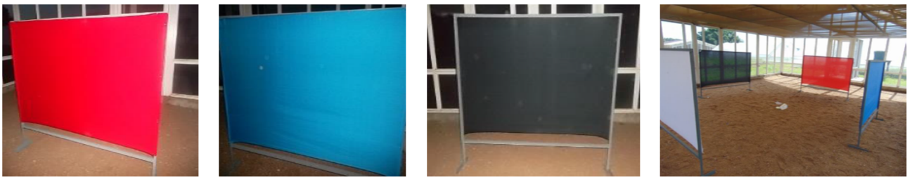
a) Red fabric anchored on a frame b) Blue fabric anchored on a frame c) Black fabric anchored on a frame d) frames arranged inside SFS, insect releasing point at the center
