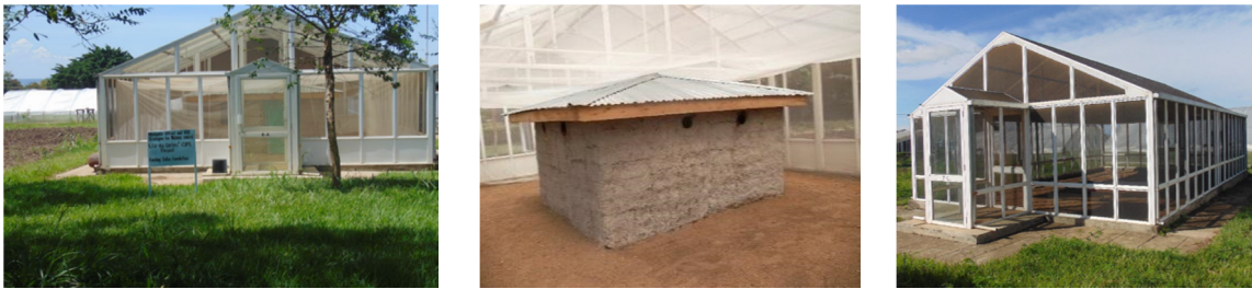
a) Semi field system(SFS) with hut inside b) Mud walled hut inside SFS c) Open SFS (No hut inside)
