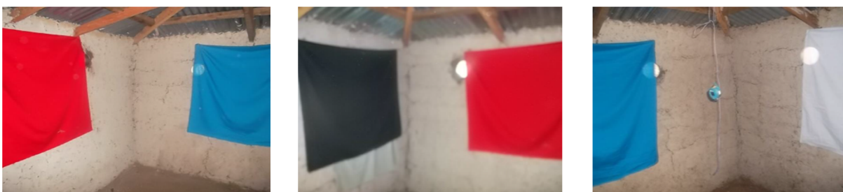
a) 1 st Section of hut walls with anchored coloured fabrics inside to create resting sites b) 2 nd Section of hut walls with anchored coloured fabrics inside to create resting sites c) 3 rd Section of hut walls with anchored coloured fabrics inside to create resting sites; Hobo data loga at the middle corner
