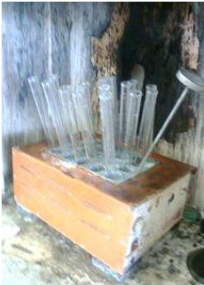
Appendix VIII Boiling tubes with samples in Kjeldhal digestion plate.
